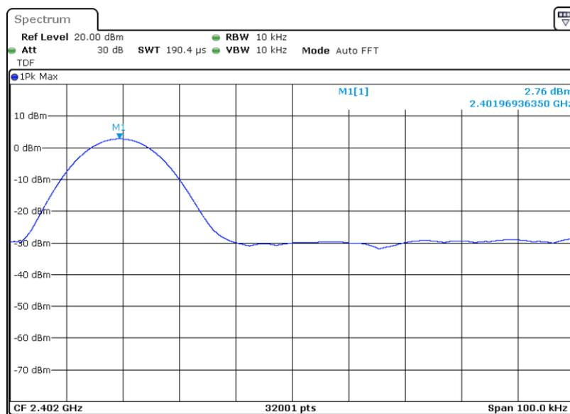
Figure 6-2 Example test plot of frequency tolerance testing
